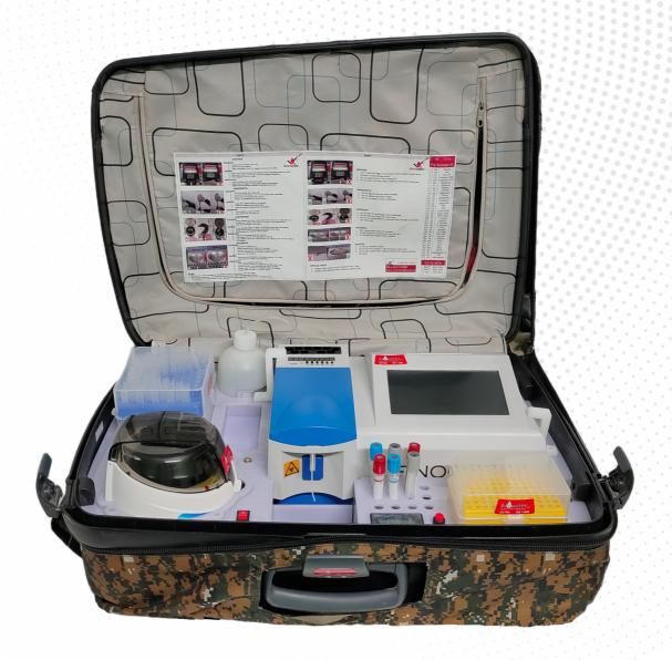
**ACLABOX-BIOCHEM** is a compact & portable clinical Laboratory with an open system Semi-Auto chemistry Analyzer in a suitcase. This is rugged & maintenance free.
