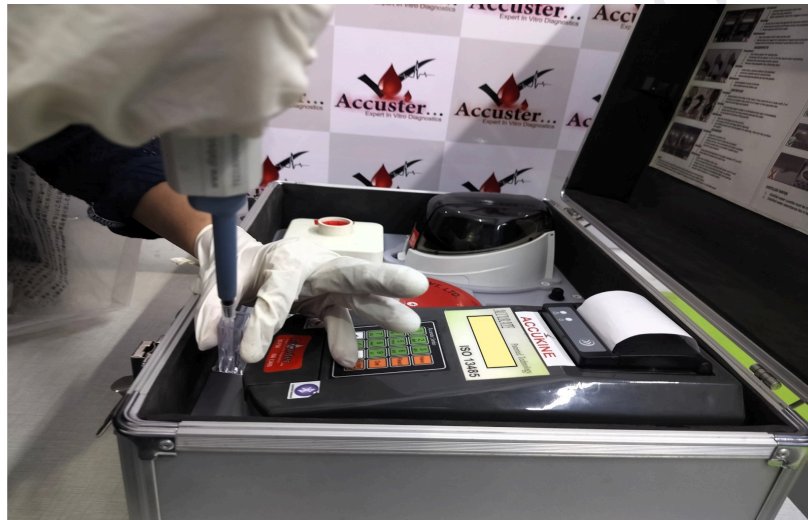
Fig.) The correct way to hold a cuvette and add a sample , along with pressing the enter button is demonstrated (All kinetic test)
